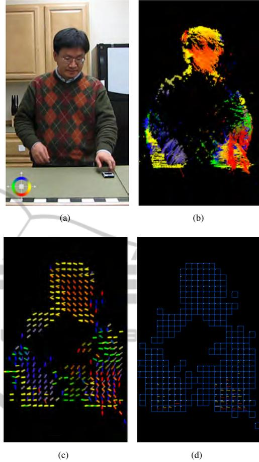
Figure 2: Direction model of an 'answerPhone' action. (a) current frame, (b) Optical flow vectors, (c) Direction model of the video sequence, (d) Magnitude model of the video sequence.
