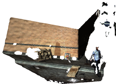
Figure 2: Textured 3D scene mesh generated from stereo disparity information from the image shown in figure 1. Notice how well the main surfaces in the scene are reconstructed.
