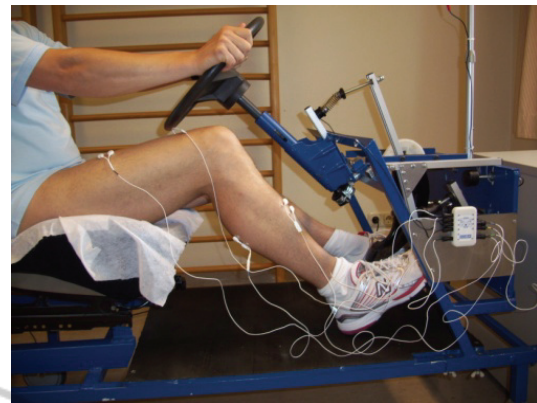
Figure 1: Car simulator with BioPlux Research system.
