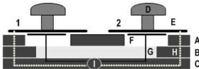
Figure 1: Cross section scheme of the double headed PZ probe. **A, B** - support layers; **C**- signal conditioning layer; **D**- 'mushroom' PVC interface **E** - PZ metal disk; **F**- PZ material **G** – PZ signal conductor **H** – ground conductor **I** – coaxial cable **1**- PZ<sub>1</sub>; **2**- PZ<sub>2</sub>.
