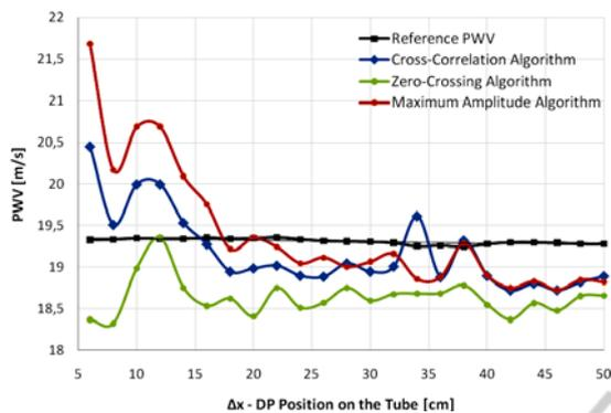
Figure 5: PWV values of unclouped PZs and pressure sensors, yielded by the three algorithms.
