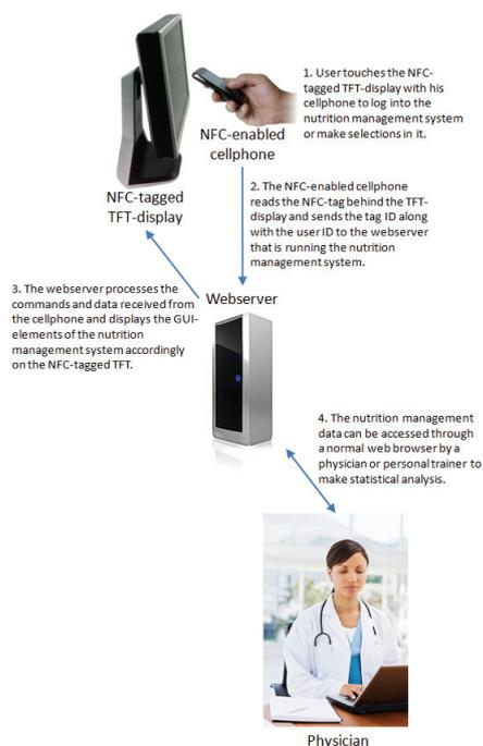
Figure 1: Interaction Process of the TnD prototype system.
