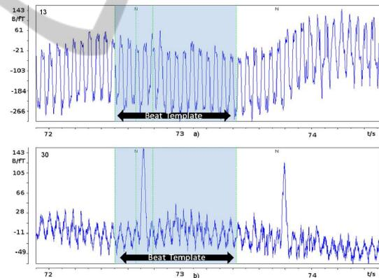
Figure 3: Raw data in two channels: a) The upper panel shows a channel with a transient vibration picked around 14-15 Hz, b) The lower panel shows a channel with very high SNR. The beat with blue background is the beat used for defining the template parameters.
