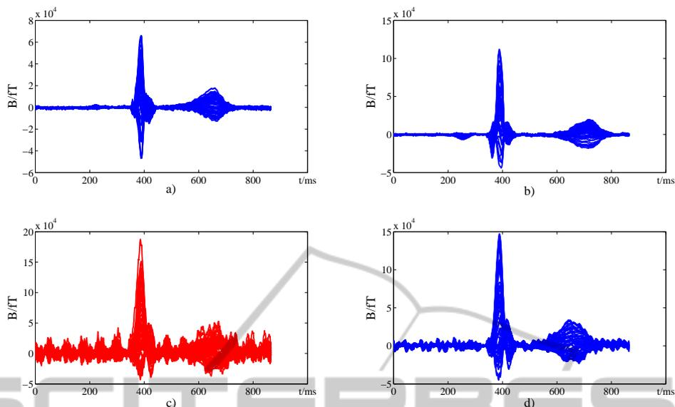
Figure 5: Averaged magnetic signals using Apollo CXS: a), b) averaged magnetic signals after CCA and transformation to standard sensor configuration (Subject 6 and 7, respectively); Subject 10 before (red) c) and after d) (blue) application of CCA and ME.
