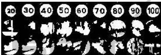
Figure 8: Binarized samples of the benchmark data set using Otsu's method.
