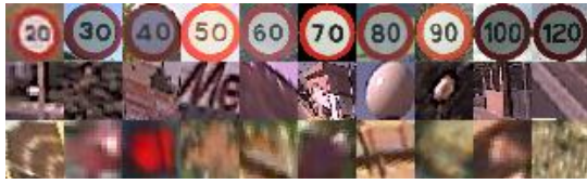
Figure 7: Examples of the benchmark data set. First row includes positive samples whereas second and third row include noisy ones.
