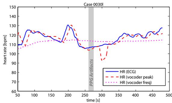
Figure 3: HR agreement comparison for Case 00301. The HR calculated by the vocoder peak method is degraded after a time offset (at 300s) when the raw PPG signal was corrupted with noise over a certain period of time (gray bar). The HR estimated by the vocoder frequency is smoothed out and does not respond quickly to large variations in HR.
