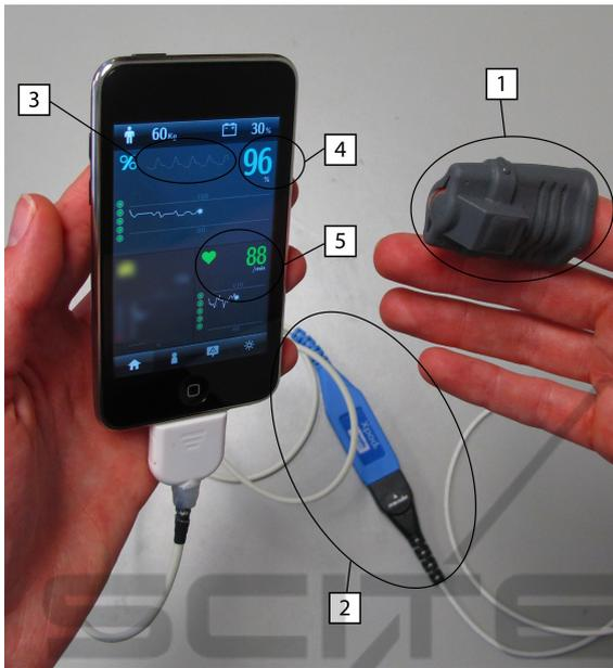
Figure 2: Phone Oximeter (Mobile phone pulse oximeter) application. 1) Soft finger probe; 2) Nonin Xpod OEM pulse oximeter module; 3) raw PPG waveform display on iPod Touch; 4) SpO2 value computed by the Xpod module; 5) HR computed by the adaptive vocoder algorithm.
