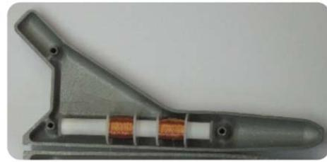
Figure 4: Electromagnetic power generator inserted inside a hip prosthesis model.
