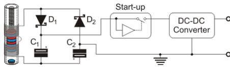
Figure 7: Energy storage and power supply circuit.
