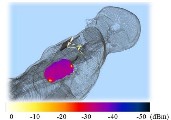
Figure 5: Example of the SAR distribution over the heart surface resulting from the exposure of the implanted phantom to the RF field generated by the birdcage coil. The two hot spots represent the contact points between the lead tips and the heart wall.
