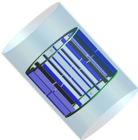
Figure 1: FDTD model of the RF birdcage coil.
