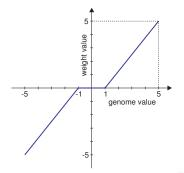
Fig. 3. Threshold function that decodes genome values into weight values, preserving sparse weight coding.
