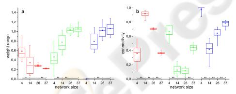
**Fig. 5.** Optimal weight range and connectivity depends on reservoir size. Network structure after full-weight optimization of the selected networks from fig.4. a) Weight range of all non-zero weights of the reservoir (red), the backprojection weights (green) and the input weights (blue). b) Connectivity (percentage of non-zero weights). Boxplots show 5%, 25%, 50%, 75% and 95% quantiles of N=20 datapoints. \* p ; 0.05; \*\* p ; 0.01.
