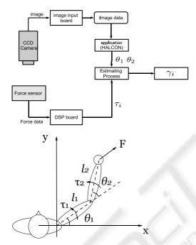
Figure 2: Schema of the experimental system and objective.
