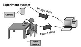
Figure 1: The experimental system.
