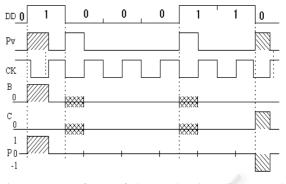
Figure 5: Waveforms of the synchronizer discrete and automatic.
