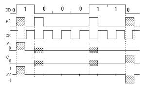
Figure 3: Waveforms of the synchronizer discrete and manual.
