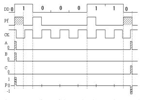
Figure 7: Waveforms of the synchronizer continuous and manual.
