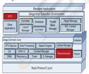
Figure 1: Ginga Middleware Architecture (adjusted with the recommendation system).
