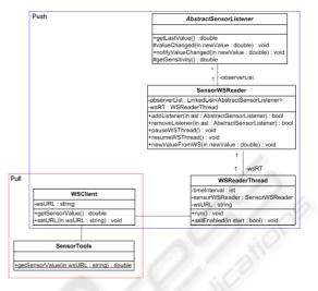
Figure 3: The Context Acquisition API class diagram.
