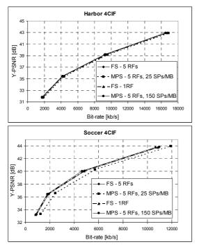
Figure 3: Rate-distortion curves for 4CIF sequences.
