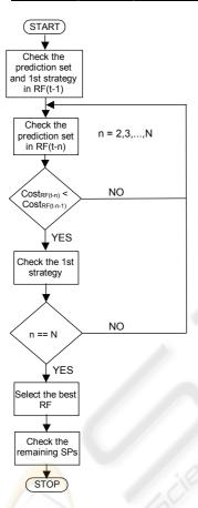
Figure 1: The flowchart of proposed MRFME method.
