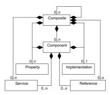
Fig. 1. A basic view of SCA meta model.
