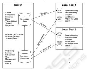
Figure 3: Collaboration between different users through a central server.
