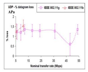
Figure 6: UDP - percentage datagram loss results versus technology and nominal transfer rate; Expa.
