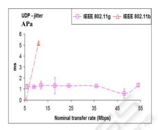
Figure 4: UDP – jitter results versus technology and nominal transfer rate; Expa.
