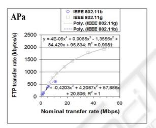
Figure 8: FTP transfer rate versus technology and nominal transfer rate; Expa.
