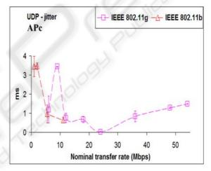
Figure 5: UDP – jitter results versus technology and nominal transfer rate; Expc.
