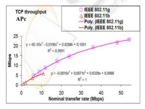
Figure 3: TCP throughput versus technology and nominal transfer rate; Expc.
