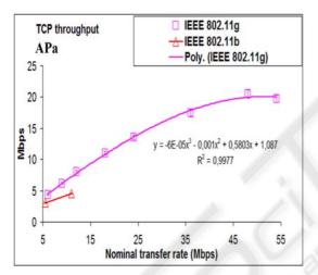
Figure 2: TCP throughput versus technology and nominal transfer rate; Expa.
