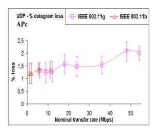
Figure 7: UDP - percentage datagram loss results versus technology and nominal transfer rate; Expc.
