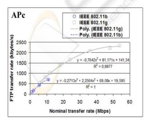
Figure 9: FTP transfer rate versus technology and nominal transfer rate; Expc.
