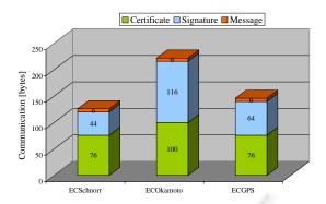
Figure 9: Communication overhead of evaluated signature schemes.
