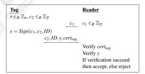
Figure 3: Entity authentication based on a signature scheme.
