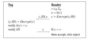
Figure 2: Entity authentication based on an encryption scheme.
