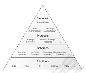
Figure 1: Different public-key techniques lead to the cryptographic service of authentication.
