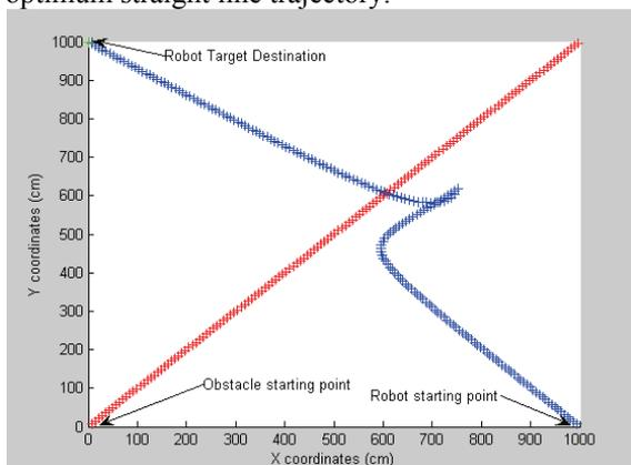
Figure 3: Standard Potential Field robot with dynamic obstacle.
