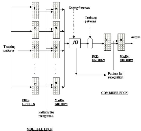
Figure 6: Schematic of the PCN based Multi-Classifier.
