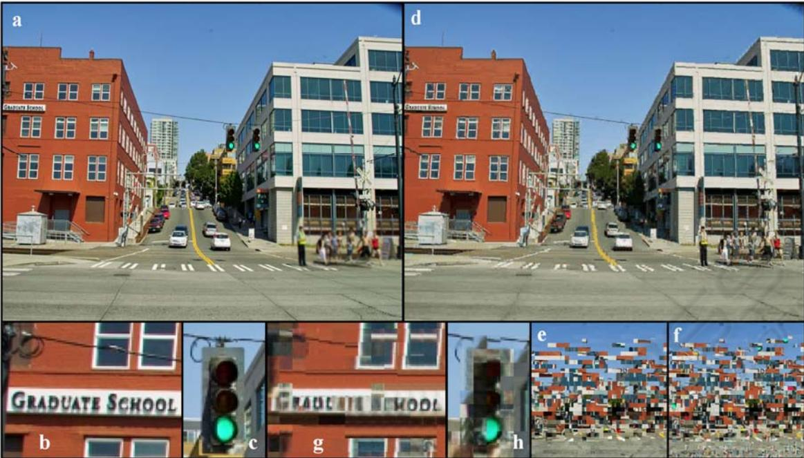
Figure 1: a) original photograph, resolution 1024x768; b) cut-out of size 110x80; c) cut-out 50x80; d) k-means clustering using random seeds; e) initial codebook (1k codevectors); f) final codebook; g) and h) cut-outs of decompressed image.
