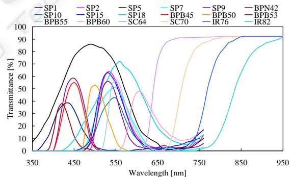
Figure 2: Transmittance of filters.
