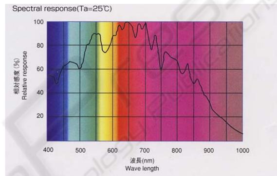
Figure 1: Spectral sensitivity of line CMOS camera.
