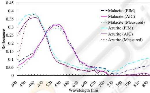
Figure 7: Representative result of spectral reflectance reconstruction.
