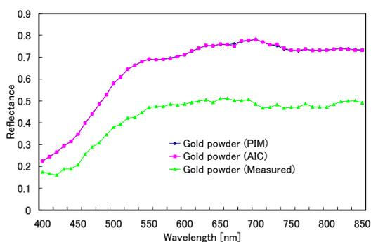
Figure 9: Spectral reflectance reconstruction of glossy target.
