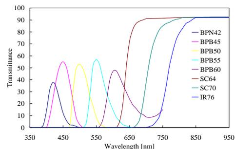
Figure 6: Transmittance of selected filter.
