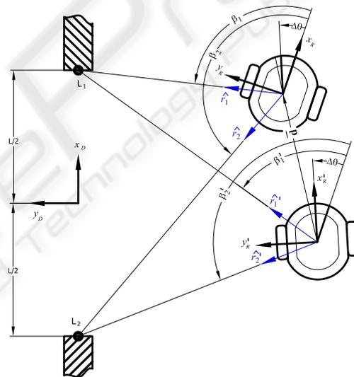
Figure 4: Robot position from bearing.
