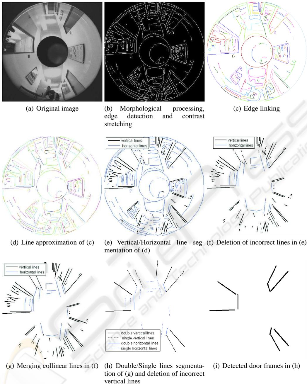
Figure 2: Overview of image processing steps in door detection.
