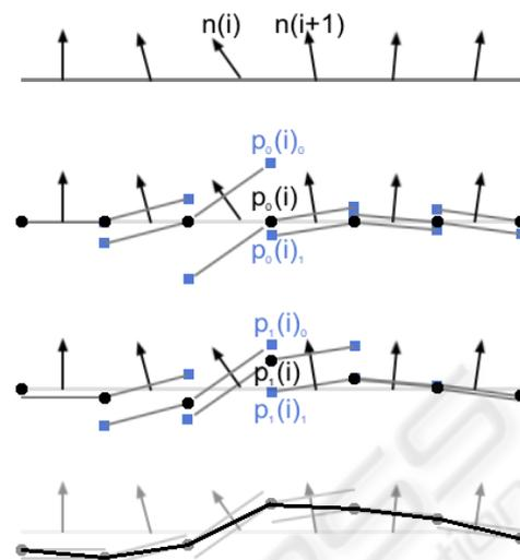
Figure 3: An illustration of our surface reconstruction algorithm as applied to a 2D normal map. The black circular dots represent the current positions, while the blue square dots are where the neighboring texels at their current positions require the positions to be. Please note that all 2D normal maps in fact correspond to valid 2D-surfaces (ie. piecewise linear functions), which is not the case with all 3D normal maps.
