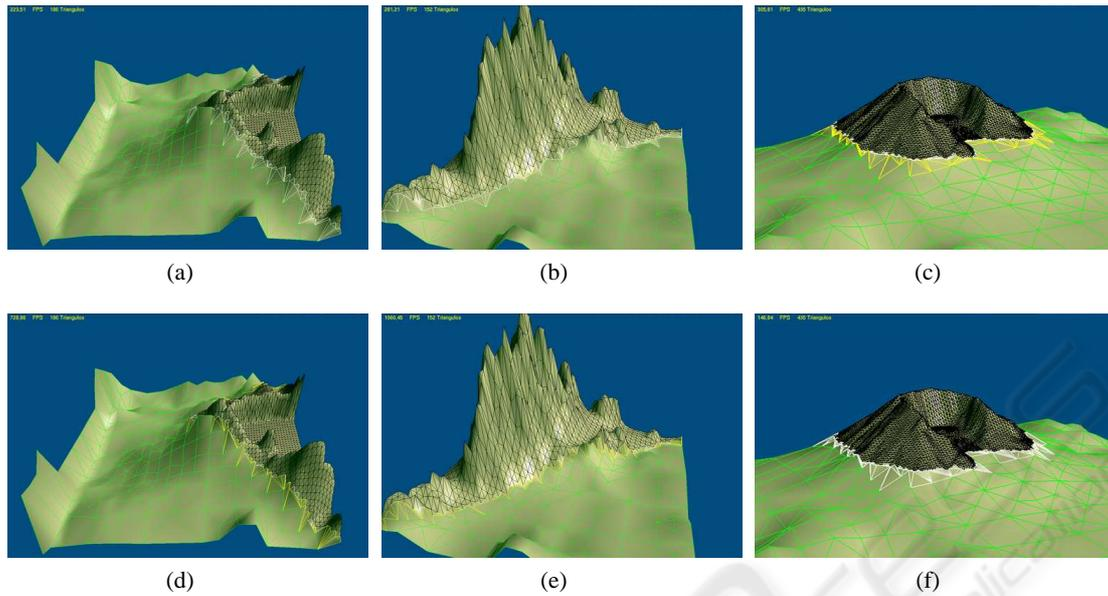
Figure 4: Adaptive tessellations generated by both proposals. Subfigures (a), (b) and (c) are generated by the proposal based on the incremental randomized triangulation. Subfigures (c), (d) and (e) are generated by HM based proposal.
