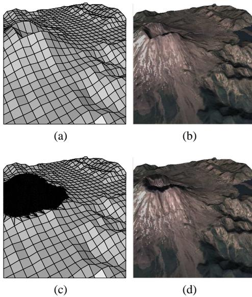
Figure 1: Hybrid terrain model. (a) Grid (b) Grid with texture (c) Hybrid model (d) Hybrid model with texture.
