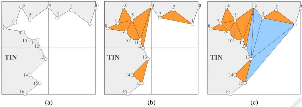
Figure 3: Four cells of a grid with the TIN silhouette. (a) Before convexification (b) Finest LOD level convexification (c) Coarser level convexification.
