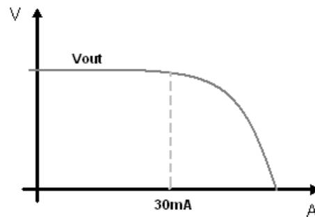
Figure 12: Output voltage versus current. For currents above 30mA the system protection responds by reducing the output voltage.
