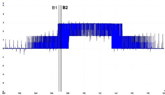
Figure 7: Signal obtained at the output of the H-Bridge circuit, with 2s in time axis and 5V in voltage axis.
