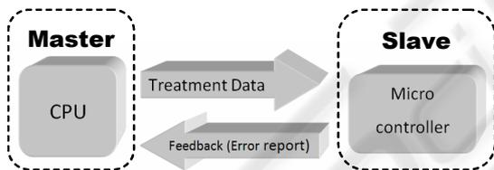
Figure 3: System architecture. The CPU operates as master and the micro controller operates as slave. The micro controller functionalities are controlled by the CPU.
