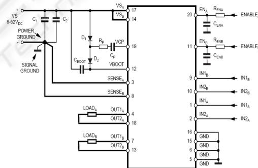
Figure 6: H-Bridge circuit based on BCD technology. Combines isolated DMOS Power Transistors with CMOS and bipolar circuits on the same chip.
