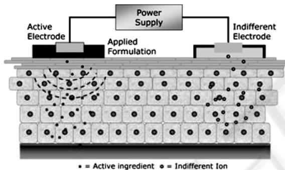
Figure 2: Electric field generated by the electrodes. It is visible the response of cream particles along the hypoderm.
