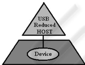
Figure 5: Reduced Host Topology. A reduced host controller has a unique USB port and does not handle full USB tree with hub. It means that a reduced host controller is designed to handle a unique point-to-point connection with an unique USB device.
