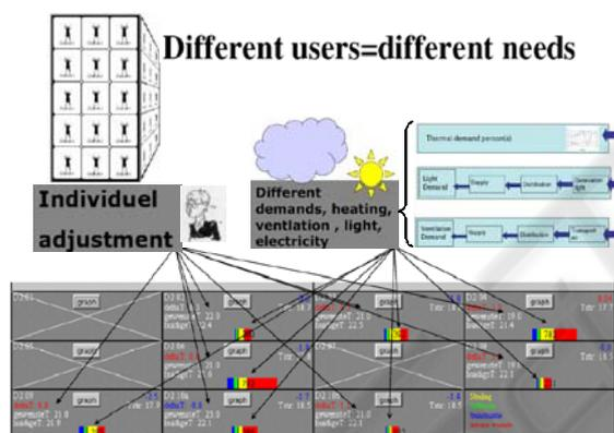
Figure 1: Individual adjustments and different energy demands for each office room shown on the screen of the BMS (Hommelberg 2005).
