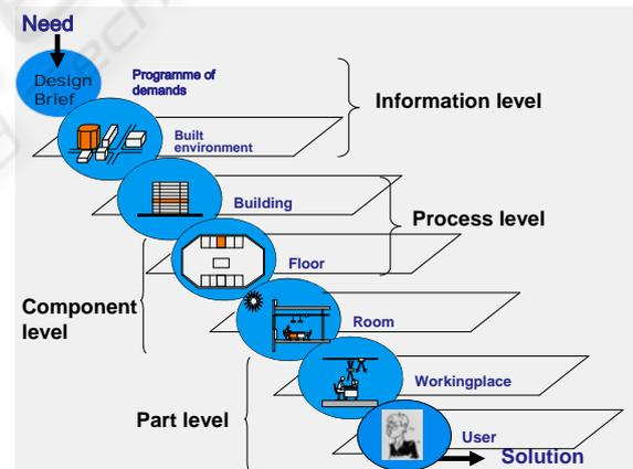
Figure 4: Hierarchical abstraction levels by functional decomposition.
