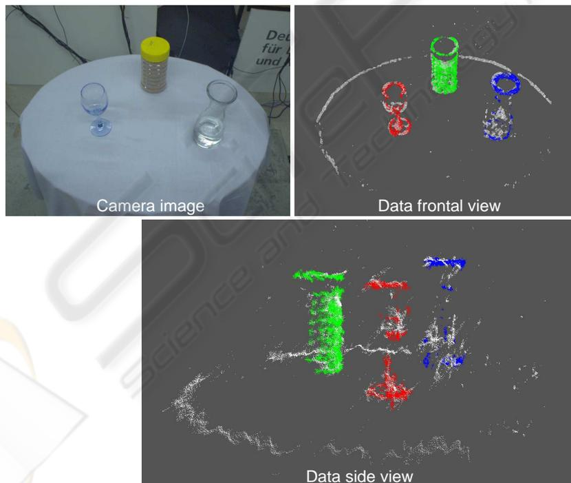
**Fig. 2.** Scene with objects used by the humanoid 'Justin' (cf. fig. 1) for preparing an instant-tea drink: camera image and stereo data points (white) superposed with model points of the recognized objects (colored).
