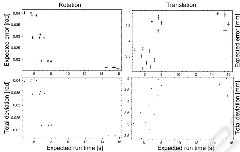
**Fig. 4.** Plots of error statistics versus run time statistics for the 16 tested variants of pose estimator: expected error  $E(\|\hat{\mathbf{p}} - \mathbf{p}_{\text{ref}}\|)$  (bars indicate standard errors of the expectation values) and total deviation  $\sqrt{\text{Tr } \mathbf{C}}$ , each for rotation and translation parameters.
