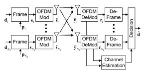
Figure 1: MIMO-OFDM baseband system model.
