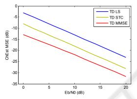
Figure 5: Channel estimation MSE (BRAN-A indoor channel).
