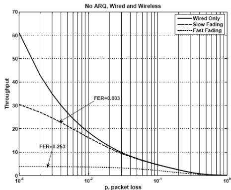
Figure: 2 Effect of air channel on TCP throughput (kbps).
