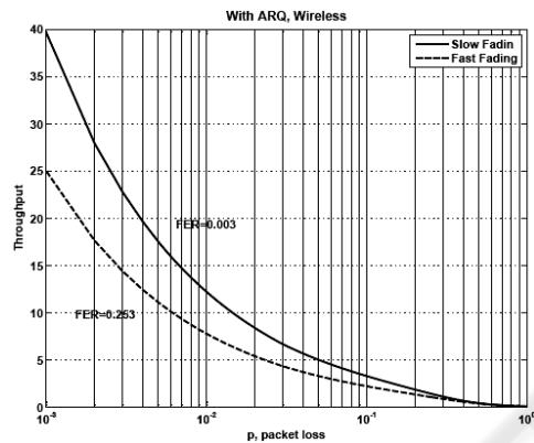
Figure: 3 Effect of air channel on TCP/ARQ throughput (kbps).
