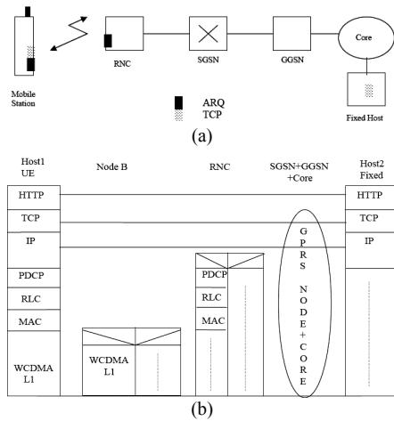
Figure 1: (a) An end-to-end system (b) The protocol stack on the way.
