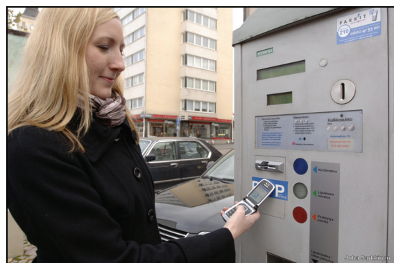
Figure 1: A user selects a parking zone by touching an NFC tag on the fare collection machine.
