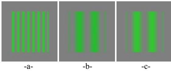
Figure 5: Example of corrected pattern. a- input stimulus at frequency  $f$ . b- stimulus at frequency  $f'$  and same color as (a). c- Spatially corrected stimulus from  $f$  to  $f'$ .
