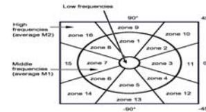
Figure 10: Decomposition in Fourier domain.
