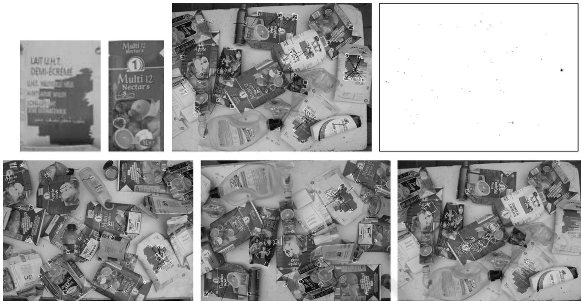
Figure 6: Some experimental results. Top row: model photos of milk and juice cartons, query image with matching visual words (white) and relative anchor locations (black) for the milk carton, hough space. Bottom row: Two query images with detected milk cartons, one with detected juice carton.
