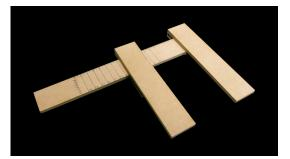
Figure 7: Self-made sliding calliper.
