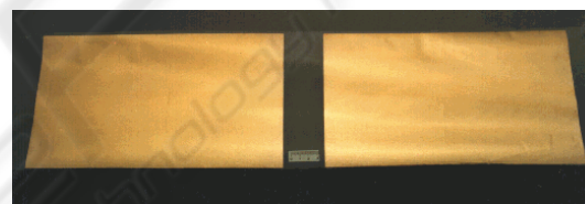
Figure 1: Metallized PVDF sheets. Piezotech S.A..
