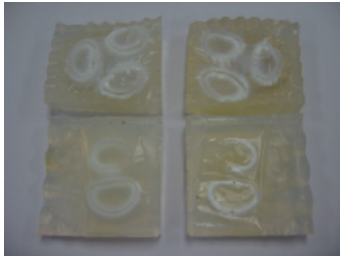
Figure 4: Silicone moulds obtained from laser stereolithographic models.
