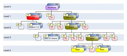
Figure 1: Structure of an XML document.
