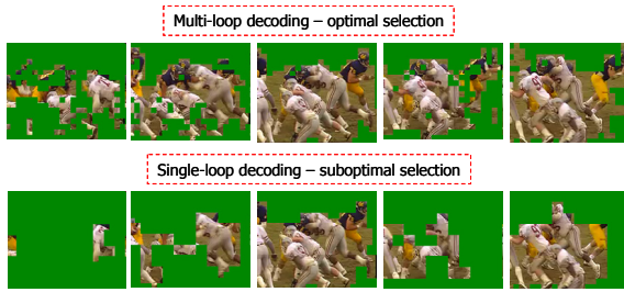
Figure 3: The intra and inter coded macroblocks in multi-loop decoding and single-loop decoding mode (green parts are the inter coded macroblocks).
