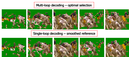
Figure 6: The intra and inter coded macroblocks in multi-loop decoding and single-loop decoding with smoothed reference prediction (green parts are the inter coded macroblocks).
