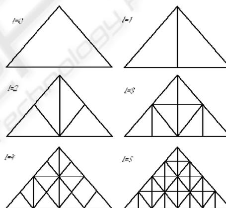
Figure 1: First 6 levels of a Binary Triangle Tree.
