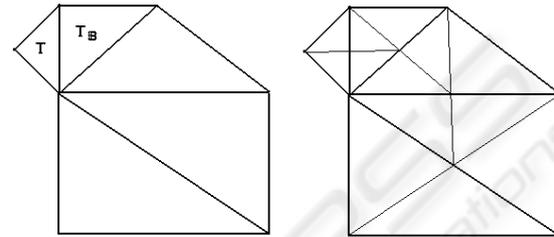
Figure 3: In order to split  $T$  all the triangles along the longest edge path have to be split first.
