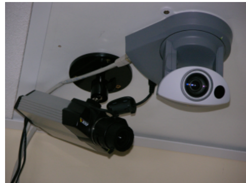
Figure 1: Our system of collocated cameras : the static camera is on the left and the dynamic camera is on the right.
