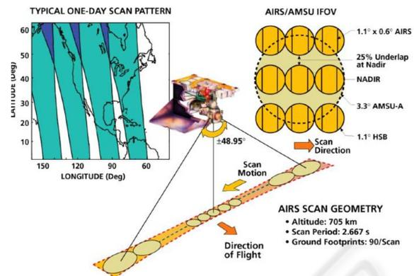
Figure 1: Cross track scan fov patterns and overlap fovs for two atmospheric radiance instruments, AIRS and AMSU currently flying on the NASA research satellite AQUA.
