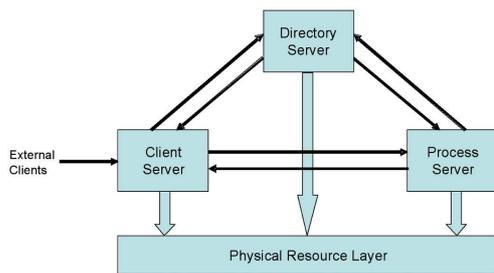
Figure 3: SOA Architecture Block Diagram.
