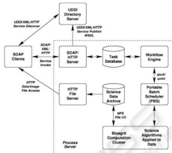
Figure 4: Internal Architecture with an independent SOAP Client.
