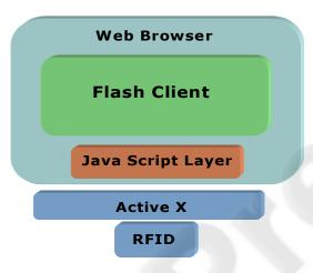
Fig. 2. Software layers in the client.
