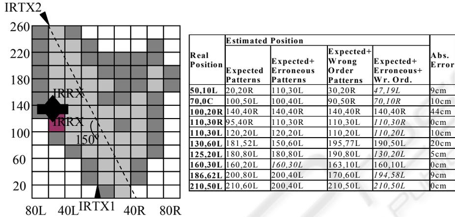
Fig. 4. Mapping of Reliable (pale shade) and Unreliable regions on the grid.
