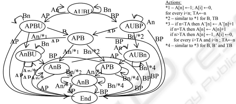
Fig. 2. FSM for the recognition of the patterns received on IRRX<sub>A</sub> and IRRX<sub>B</sub>.
