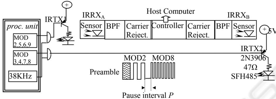
**Fig. 1.** The architecture of the IRTX and the IRRX device. A sample pattern sequence: A Preamble followed by one MOD2 and one MOD8 pattern.
