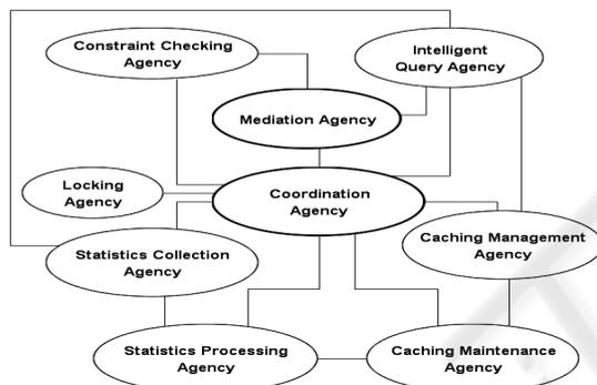
Figure 1: The architecture of the proposed data management agent-based framework.
