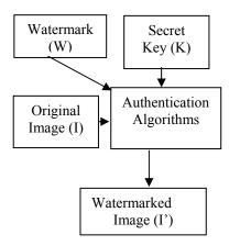
Figure 1: Block diagram of a watermark embedding system.
