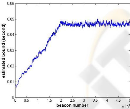
Figure 6: Estimated bound for sending 95% of the frames.
