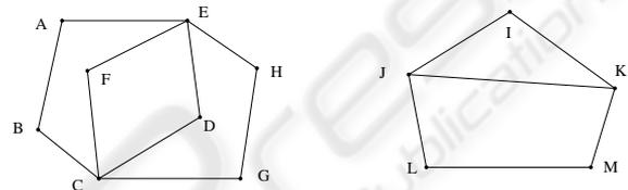
Figure 3: Non-interior-intersection constraint (left: If both  $ABCDE$  and  $HGCFE$  are 2D faces then they must be coplanar, otherwise their intersection  $CE$  must be a visible edge); Chordless constraint (right: cycle  $I J L M K$  contains a chord  $JK$ , so it is not assigned as a face, instead,  $IJK$  and  $JLMK$  can be assigned as faces).
