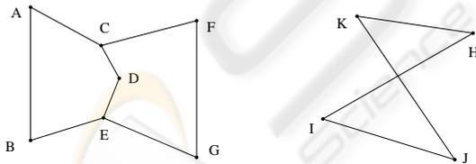
Figure 2: Face adjacency constraint (left: if both  $ACDEB$  and  $FCDEG$  are 2D faces then they must be coplanar); Non-self-intersection constraint (right: since edges  $HI$  and  $JK$  intersect not at a vertex, cycle  $H I J K$  cannot be the projection of a 2D face).
