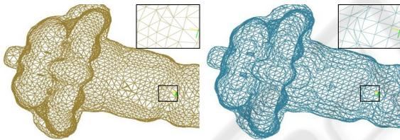
Figure 1: Better triangles in isosurface obtained using dual contouring (left) than MC method (right) for the fuel dataset (from <http://www.volvis.org>). The dual contouring result is obtained from the isosurface points computed using our method.
