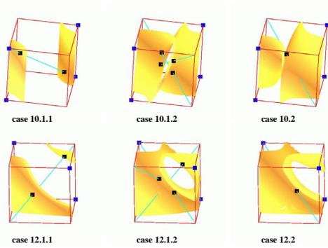
Figure 5: Topological configurations with two ambiguous faces: trilinear model in yellow-orange, isopoints in black, positive nodes in blue, rays in cyan.
