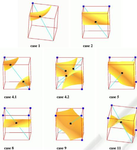
Figure 3: Topological configurations with no ambiguous faces: trilinear model in yellow-orange, isopoints in black, positive nodes in blue, rays in cyan.
