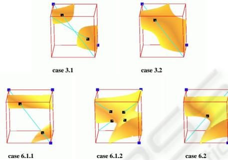
Figure 4: Topological configurations with one ambiguous face: trilinear model in yellow-orange, isopoints in black, positive nodes in blue, rays in cyan.
