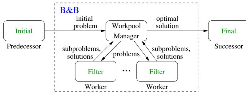
Figure 2: Branch & bound skeleton with centralized work pool manager.
