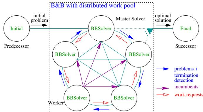
Figure 5: Branch & bound skeleton with distributed work pool.
